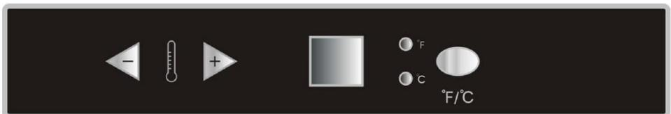
This kegerator has digital control panel located on the top of the inside of the cabinet. Pressing the temperature buttons will make the unit colder or warmer. Press the “-” button to lower the temperature by one degree. Press the “+” to raise the temperature by one degree. This unit has a temperature range of 32-46° F.
